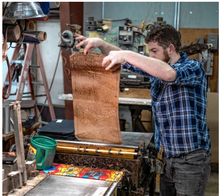
Sam Ives works on the leather cover for a family bible. Top, he cuts the leather to exact measurements. Bottom left, he adds the inlaid cross. Bottom right, he puts the leather through a glue roller to adhere to cardboard to make the cover.
